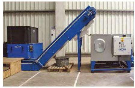
GAZ 82 S in combination with conveyor belt and briquetting press
