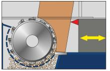
Rotor with 348 mm diameter = high material removal rate due to large wrap
